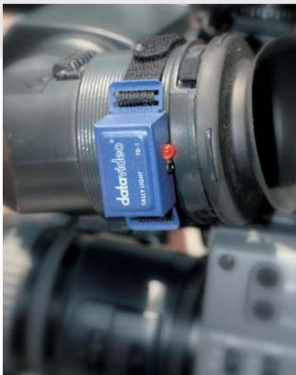
Good communication is vital in any production studio, keeping communication between the director, cameramen, lighting and control room is essential to produce a polished end result. The Datavideo ITC-100 Intercom system provides 8-Way talkback and tally indicators. The producer can select to talk to an individual channel or to all channels simultaneously.
