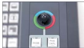
Joystick for RGB control or PiP position
