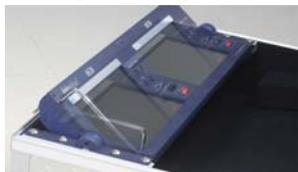
Easy adjustment of the viewing angle of the high quality TLM-702 TFT LCD monitor.
