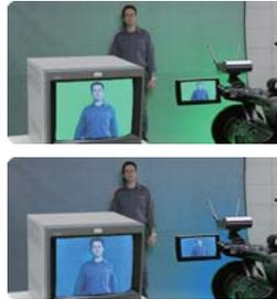
Change chromakey setup from Green to Blue with a flick of a switch on the supplied LD-1 controller
