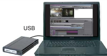
USB interface for connecting with PC or MAC based computer NLE systems
