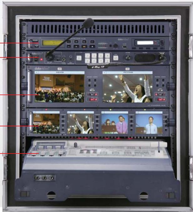
At the heart of the MS-800 lies the SE-800 4 channel DV / analogue audio video switcher. The SE-800 allows four channels of digital or analogue video and up to six channels of audio to be mixed / switched.
