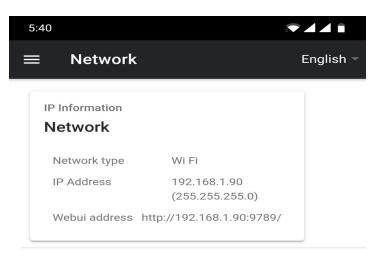
2. Open the settings menu on the slave device, enable slave mode and enter the IP address of the master.
