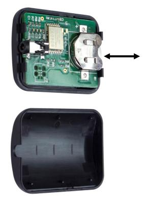
This button battery can be replaced by the user when it dies. **Please remove the back case cover carefully** to avoid user damage to the PCB or case. Then slide the old battery out.
