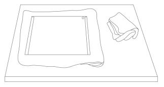
Once finished re-install the glass back into the prompter hood, again using the cloth covered edges only. *Ensure the green circle sticker on the glass is facing you* and the red circle sticker is facing the camera lens. Reseat/secure the camera hood if necessary.
