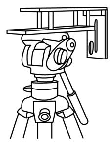
1. Attach/screw the tripod camera quick release plate to the screw holes on the base of the prompter frame, **item A**.
