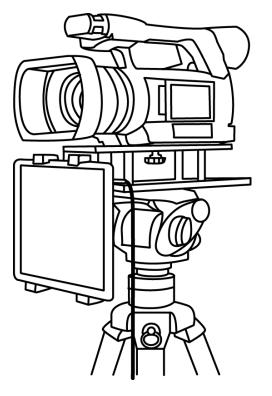
Put the configured tablet into the mounting bracket, item E, and ensure it is held securely by adjusting the size of the bracket holders for a snug fit and locking them in place. Use locking lever on item E.
