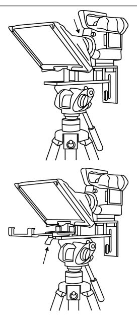
Pull the draw cord to secure the black camera Snood / Hood around the camera lens and to shut out light from camera side.
