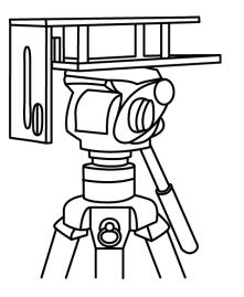
Attach/screw the tripod camera quick release plate to the screw holes on the base of the prompter frame, item A. If necessary use the adaptor screw, item C. Slide and secure the tripod plate, with prompter frame on top, onto the head of tripod. Ensure the vertical plate of the prompter frame is facing toward the on screen talent / commentator.
