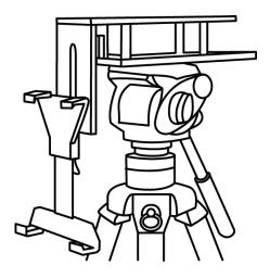
2. Use the mounting bracket screw, **item D**, to secure the mounting bracket for the tablet computer to the front of the Prompter frame's vertical plate.
